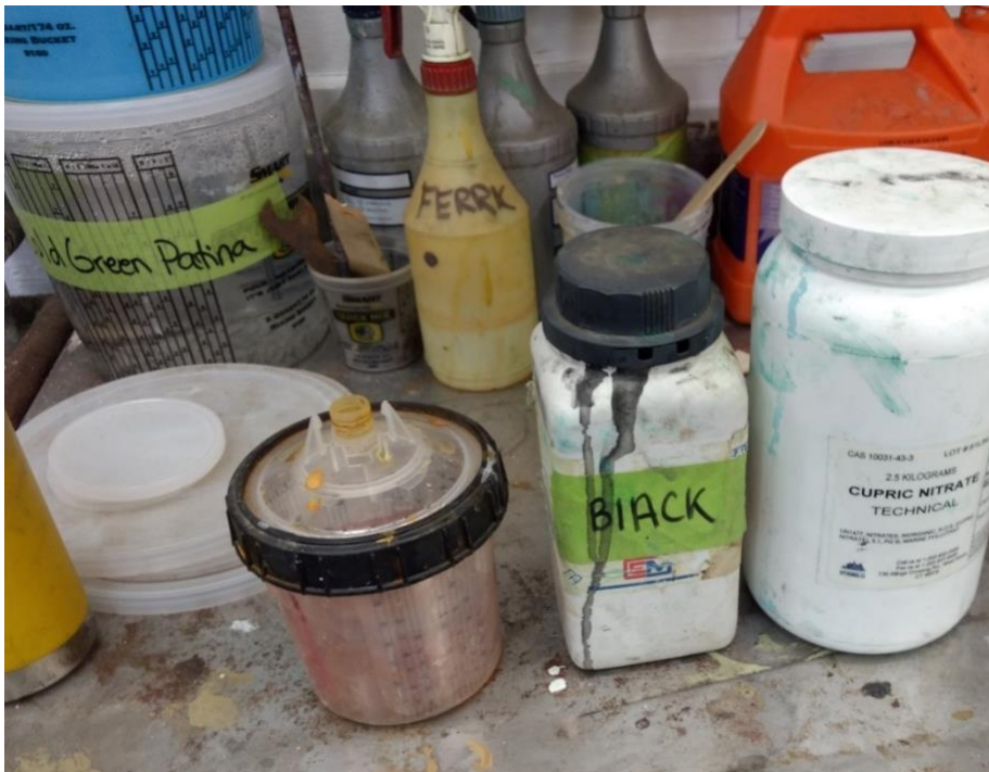
Figure 4: An image showing five examples of labeling patination reagents, with various degrees of specificity. From left to right: a) a bucket label describing method (cold) and color (green); b) an unlabeled cup whose contents the technician keeps in their memory or on the project's paper documentation; c) a spray bottle labeled with its chemical composition (ferric [nitrate]); d) a plastic bottle only labeled with its color (black); and e) a plastic bottle of powdered reagent, not yet dissolved, with the supplier's label showing all information. Image taken at The Seward Johnson Atelier by the author.
