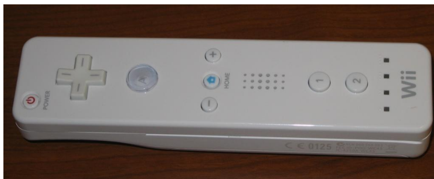
Figure 1. Photo of a Wiimote. The 3-axis accelerometer is to the left of the A button.
