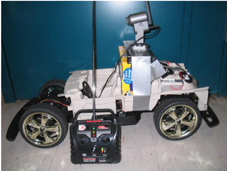
Figure 1. The camera-mounted robot and its remote control.
